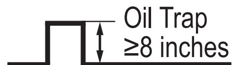
Figure 7: Close Up of An Inverted Oil Trap.
